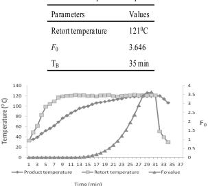
Figure 1. Heat penetration characteristics and F<sub>o</sub> value
